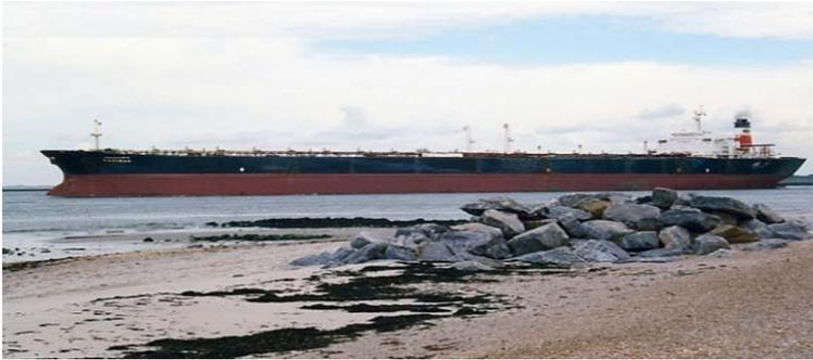
The VLCC BW Ara is a conversion candidate earmarked for future FPSO projects. The vessel is built in 1982 and has a storage capacity of 2 million barrels.
